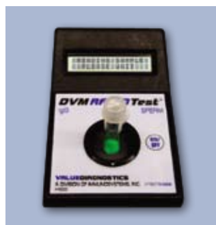
Figure 2. A commercial turbidimetric immunoassay, DVM Rapid Test™, VDX Inc, Belgium, Wisconsin, USA
