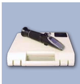
Figure 1. Sugar/ Brix refractometer 0-32%, Technika, Scottsdale, Arizona, USA
